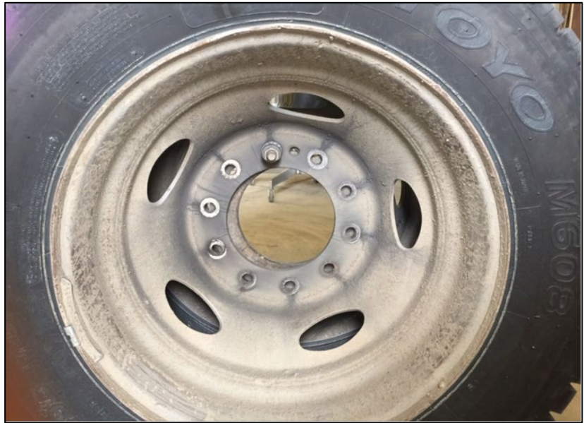
Wheel showing wear from loose lug nuts. Notice that one stud stayed connected to the wheel.
