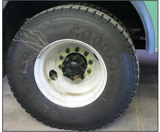
Loose lug nut indicators installed on Engine #2.
