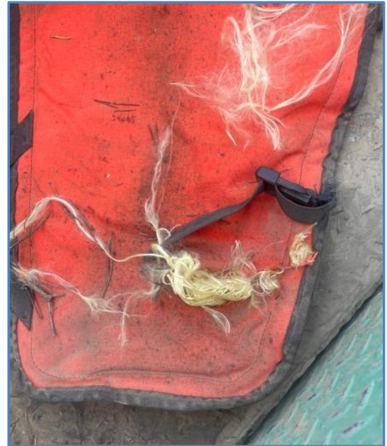
The chainsaw's saw tip kicked back, cutting into the swamper's chaps (see above), gashing a four-inch laceration into the swamper's left leg that required ten staples to close.
